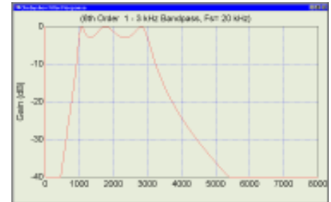
Chebyshev bandpass filter response obtained by computing the FFT of its impulse response.
