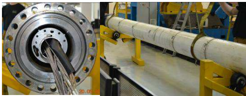
Figure 2. Electrical heater installed at inside of the pipe
