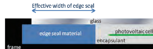
Figure 1. Schematic view of edge seal (not to scale)
