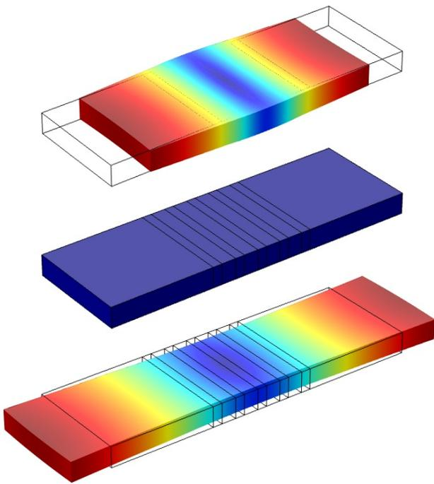
**Figure 1:** Simulation of displacement at first resonance mode 53.0 kHz at phase  $0^\circ$  (top),  $90^\circ$  (middle) and  $180^\circ$  (bottom). Displacement is scaled by a factor of  $10e8$ .
