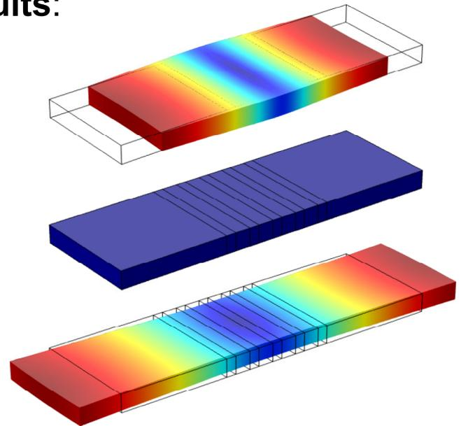
**Figure 3.** Displacement at first resonance mode.
