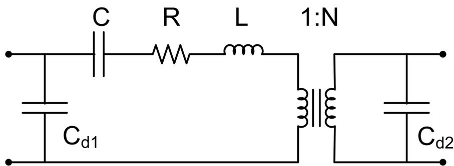
**Figure 2.** Electric equivalent circuit of a piezoelectric transformer. Only valid around a single resonance frequency.
