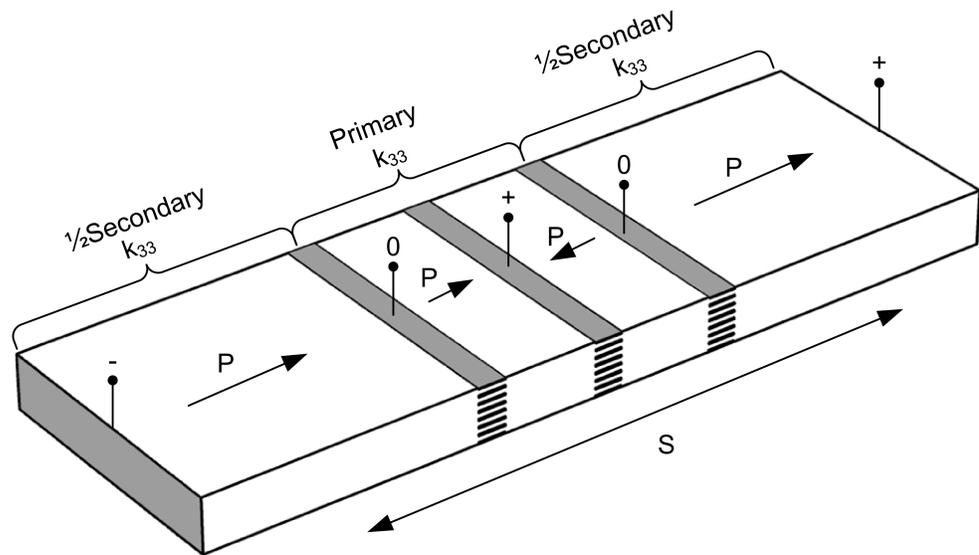
**Figure 1.** Piezoelectric transformer design: IDE Interleaved thickness mode.
