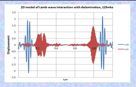
The reflected signal of A<sub>0</sub> mode is much more and can be used for detection of the damage
