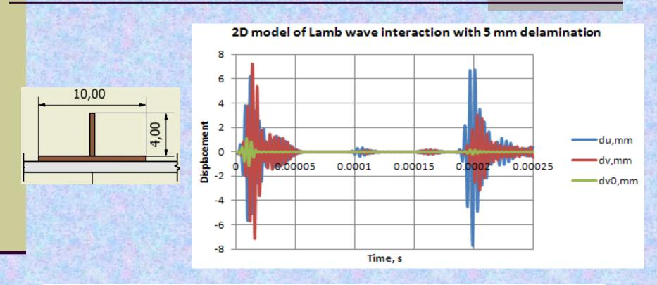
du defines the S<sub>0</sub> mode of reflected signal (blue line), dv defines the A<sub>0</sub> mode of signal that reflected from damage (red line), and dv0 defines the A<sub>0</sub> mode of a wave at initial shape of transducer (yellow line) without vertical part.
