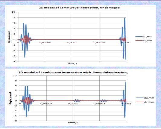
It can see the two weak signals were received by sensor before occurrence of the S0 mode reflected signal. It is reaction to delamination in composite.
