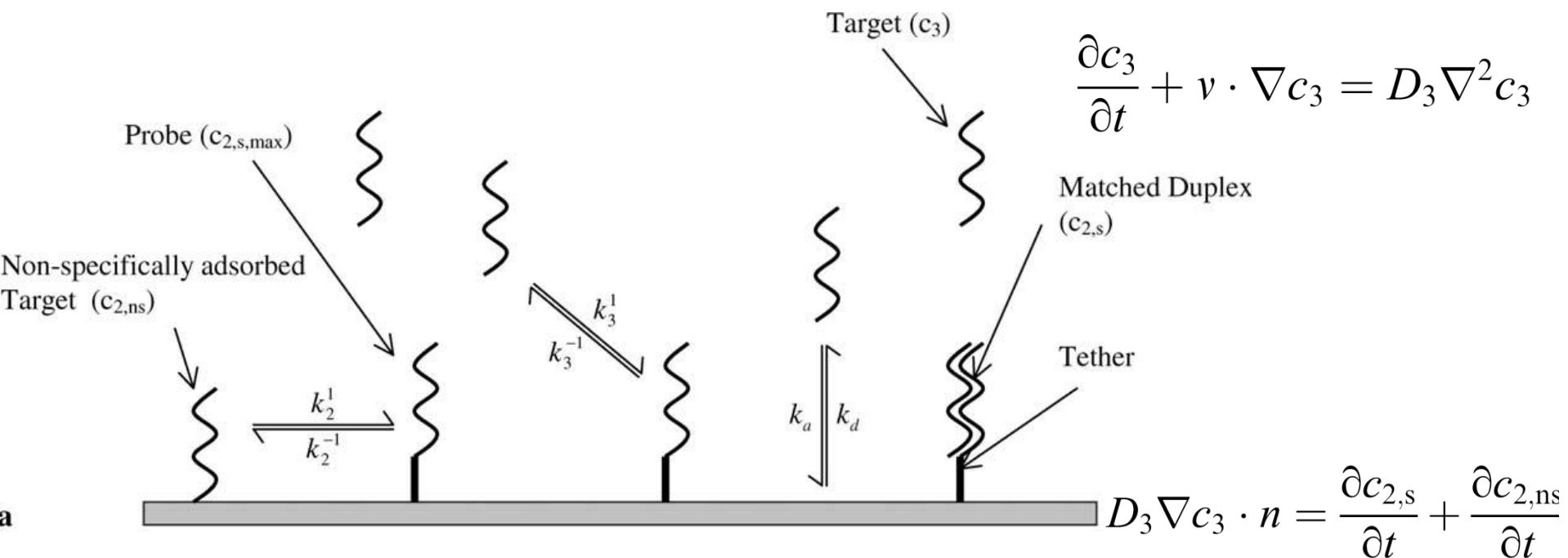
$$\frac{\partial c_{2,s}}{\partial t} = [k_3^1 c_{3,m} (c_{2,s,\max} - c_{2,s}) - k_3^{-1} c_{2,s}] + [k_2^1 c_{2,ns} (c_{2,s,\max} - c_{2,s}) - k_2^{-1} c_{2,s}],$$
