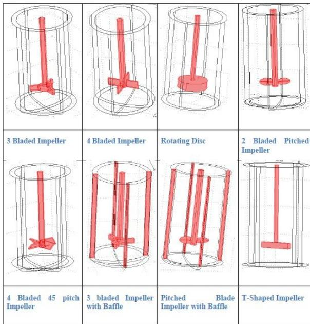
**Figure 1:** Different types of impeller geometries.
