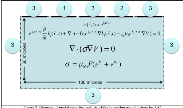
Figure 2. Diagram of model used for analysis of the logarithm model driven by A/C electric potentials.
