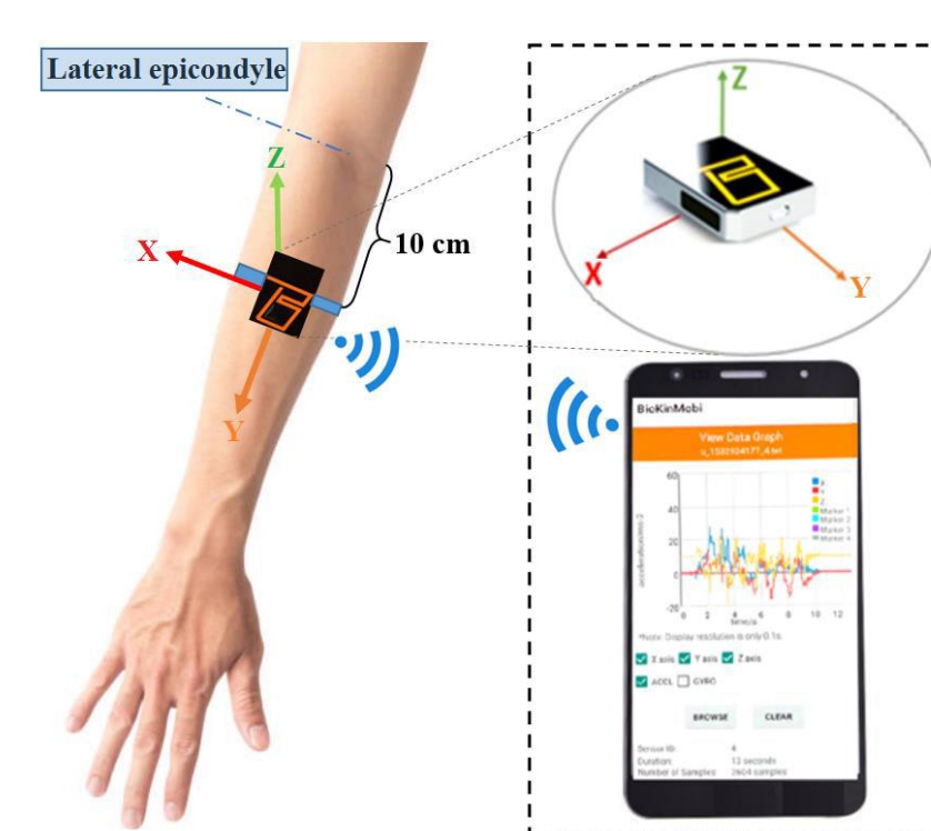
Figure 1. IMU placement can detect the shoulder motion[2]
