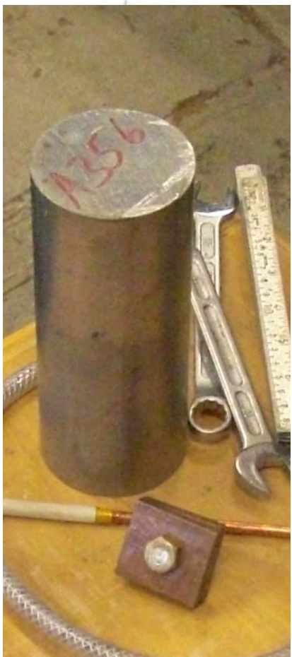
A356 aluminium alloy 48% IACS conductivity
