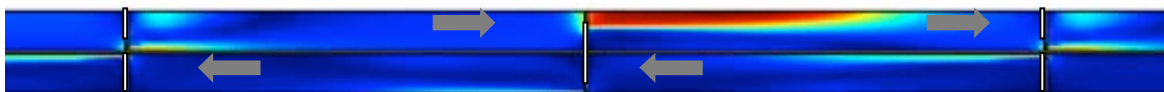
Figure 4. Velocity surface plot of the three baffle arrangement showing flow turning (Baffles in white and direction of the flow indicated by the gray arrows).
