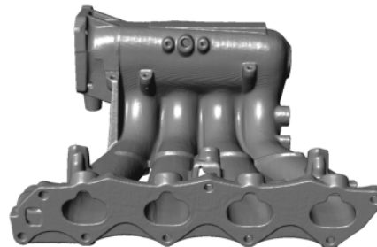
Figure 3. Segmented geometry of the solid structure of the engine manifold from the 3D CT data.
