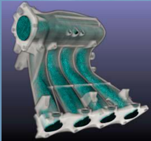
CFD mesh internal fluid structures (blue) within the engine manifold (transparent grey)
