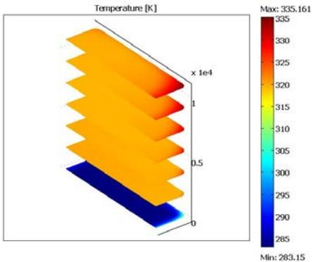
**Figure 3.** Time evolution of potato temperature during drying ( $T_a = 70^\circ\text{C}$ ,  $H = 30\%$ ,  $u_0 = 2.2 \text{ m/s}$ ).
