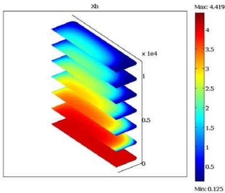
**Figure 2.** Time evolution of potato moisture content during drying ( $T_a = 70^\circ\text{C}$ ,  $H = 30\%$ ,  $u_0 = 2.2 \text{ m/s}$ ).
