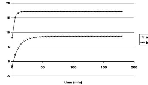
**Figure 4.** Time evolution of a and b Hunder parameters during drying ( $T_a = 70^\circ\text{C}$ ,  $H = 30\%$ ,  $u_0 = 2.2 \text{ m/s}$ ).
