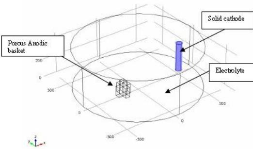
**Figure 2:** Geometrical model of ATER for copper electrorefining
