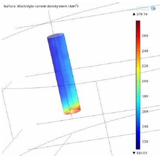
**Figure 3:** Current density distribution around the cathode
