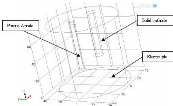
**Figure 1:** Theoretical model of lab scale copper electrorefining
