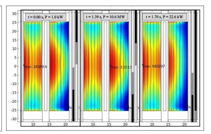
Power shifts to the OFE during control cylinder ejection and then back to IFE during safety plate insertion.
