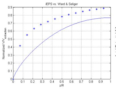
Comparison of iEPS (line) and Ga<sup>+</sup> extraction region (asterisk) normalized potential w.r.t. extraction grid voltage
