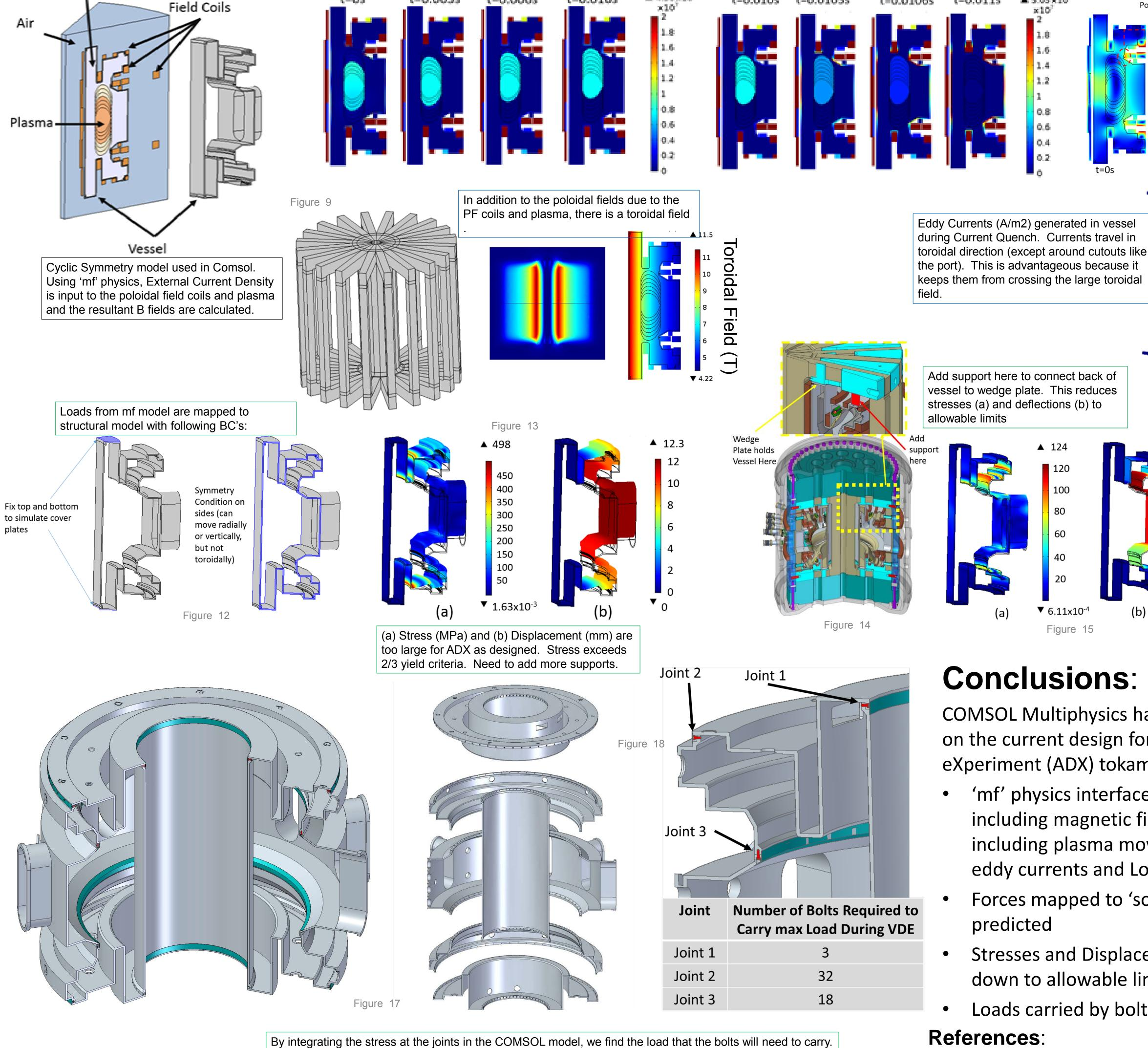
The Grade 8 bolts will be preloaded to 90% yield. 32 bolts will be able to carry the max load predicted by
