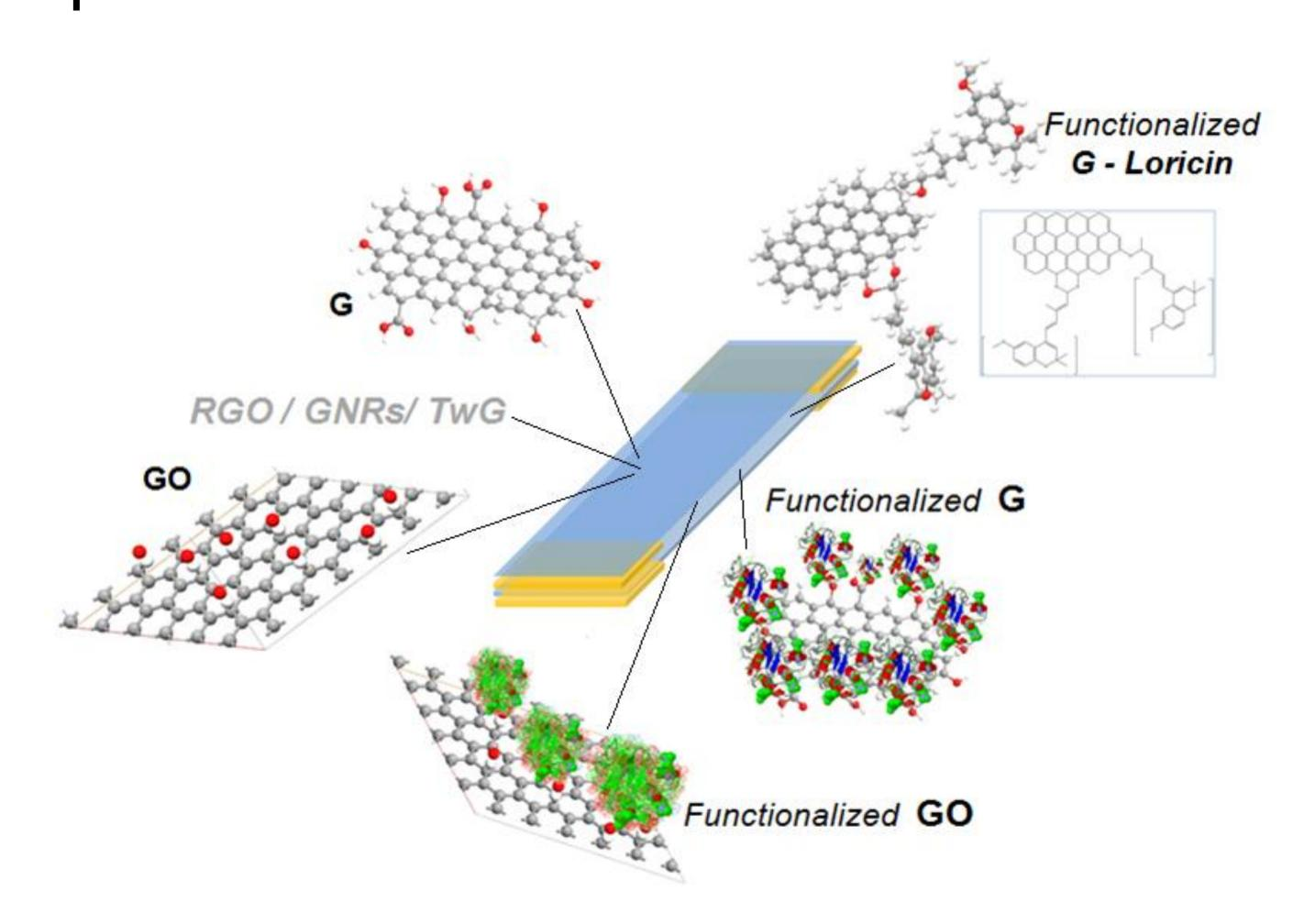
Figure 1. Basic and functionalized graphene structure models (ChemBio 3D Ultra®)
