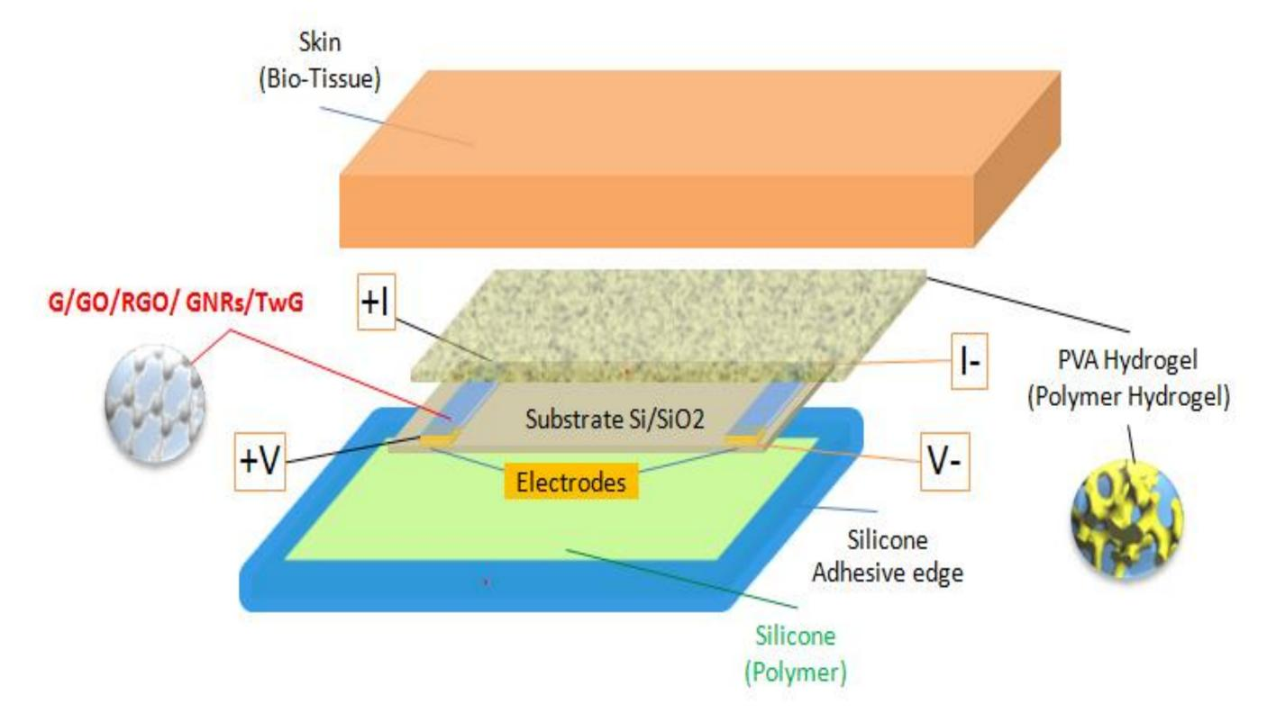
Figure 3. Multilayer graphene sensing device
