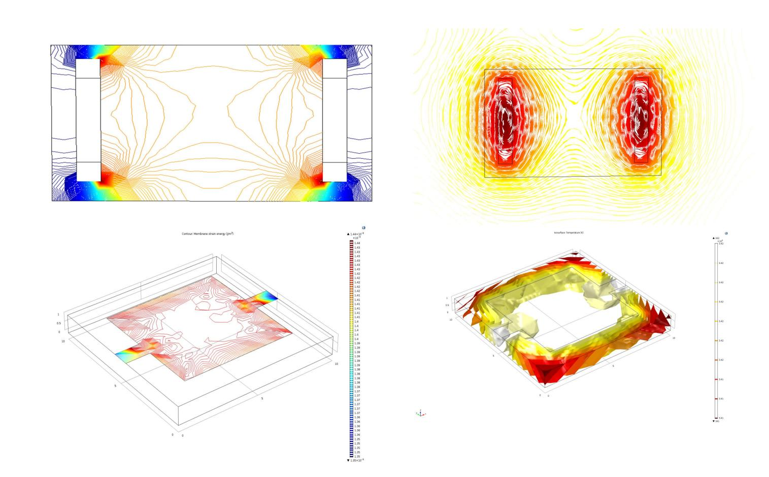
Figure 4. Electric potential (a) 2 electrodes device; (b) 4 electrodes device
