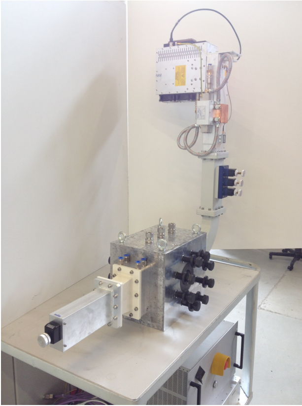
Figure 1: Applicator with magnetron head, manual tuner, aluminum block and silicon nitride tube
