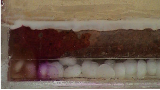
Figure 9. Phenolphthalein color change to violet in the sodium hydroxide layer.
