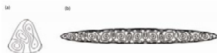
Figure 9: Streamline plot of velocity field for a keyhole shaped cavity (a) and for an elliptical shaped cavity (b) at Ra=1E6 with laminar flow assumption
