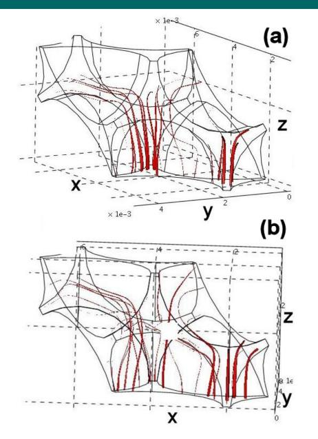
Rhombohedric unit pore cell: inlet pressure at the bottom and zero pressure boundary at outlet faces.
