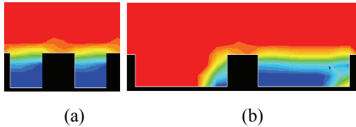
Fig. 9 Volume fractions of air and water for a=c=30\mu\text{m} , V_i=0.045\text{m/s} (a) b=30\mu\text{m} (b) b=90 \mu\text{m}
