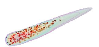
**Figure 1**: Carbide particles inside a laser cladding melt pool.
