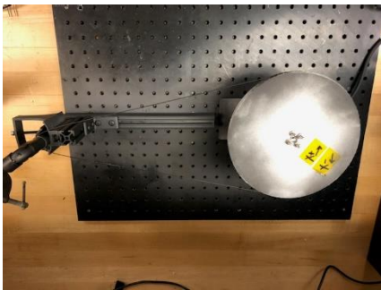
Figure 1. Army Research Lab Elastocaloric Refrigeration Loop
